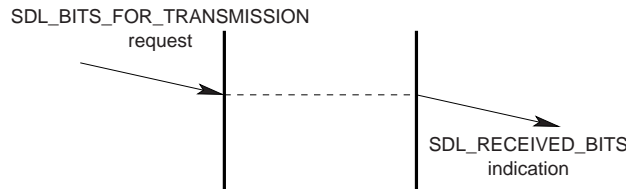
Figure 3.13: Message Flow: Successful Data Transfer Service
